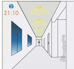
Light dims to stand-by level after the hold-time (no motion).
