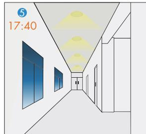
Light turns on 10% automatically when natural light is insufficient.
