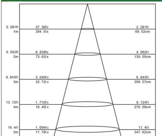
HT EAVG/EMAX ANGLE:38.34DEG DIA
