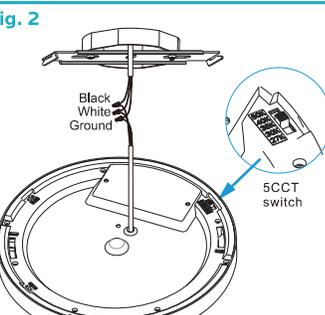
2. Wire Connections: Connect the house ground wire to the fixture ground wire; connect the white supply wire to the white fixture wire; connect the black supply wire to the black fixture wire by using the wire connectors. Carefully tuck all wires back into the Junction Box. Adjust the 5CCT switch ( See Fig.2.)
