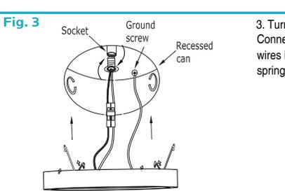
3. Turn E26 adapter into socket base. Connect Quick Connectors Tuck all wires into recessed can. Squeeze springs and push up into recessed can.
