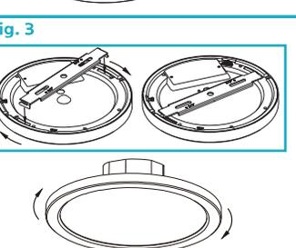
3. Snap and fix the clip in the bracket. ( See Fig . 3)
