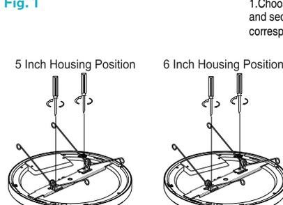
1. Choose a 5-inch or 6-inch housing and secure it with screws at the corresponding holes on the bracket.
