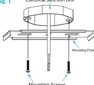
1. Pull the supply wires and house ground wire from the Outlet Box. Position the mounting plate over the Junction Box. Mark the location of the two holes located on the Mounting Plate. Be sure to mark only the narrow parts of the hole. Removing Plate from the ceiling. Drill the two holes using the appropriate type and size drill bit. Insert anchors into the holes. ( See Fig.1)
