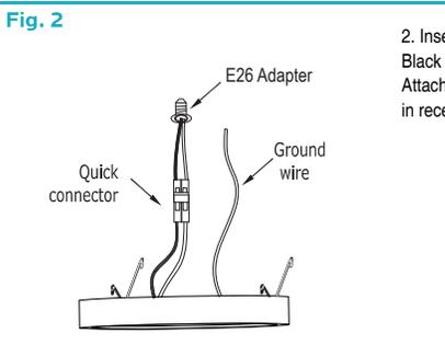
2. Insert wires into Quick connector. Black to black and white to white. Attach ground Wire to ground screw in recessed can. Adjust 5 CCT Switch.
