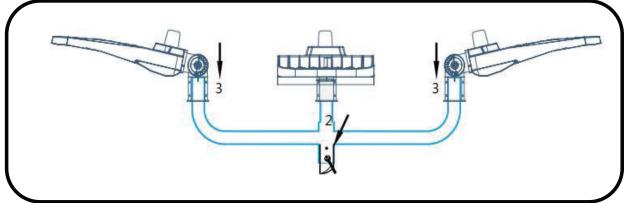
1.According to the hole position on the bracket. Draw the position on the square pole.
