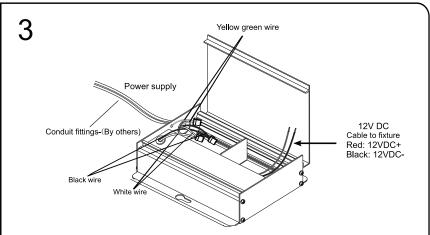
Install the included strain relief bushing in the appropriate hole then push the wires through the connector. Make connections in the compartment: match the white wire from the line feed with the white wire from the LED driver, match the black wire from the line feed with the black wire from the LED driver with the included wire connectors, match the copper wire from the line feed with the green wire from the LED driver
