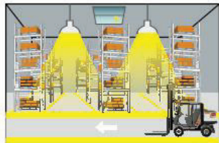
② Motion detected, lamp automatically lights up to 100%.
