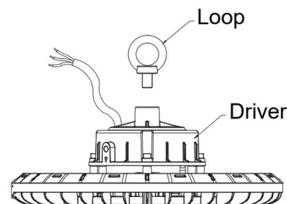
1. Screw the Loop completely into the driver hole.
