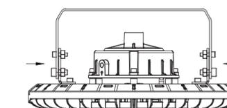
2. Screw the bracket onto the bracket fixing plate.
