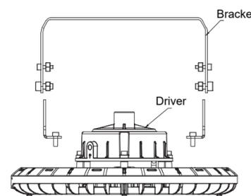
1. The bracket fixing plate is screwed to the lamp.
