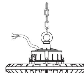
2. Hang the jack chain on the Loop of fixture
