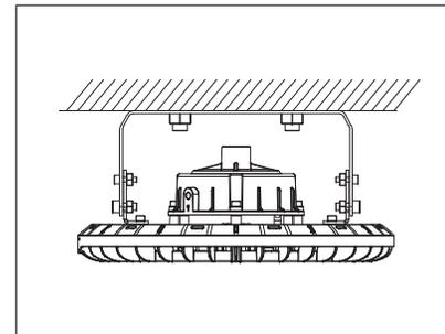
3. Install the lamp bracket on the prearranged wall screws and tighten the nuts.
