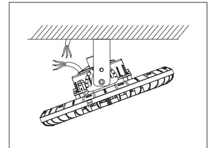
4. Adjust the proper angle of lamp, tighten the nut and connect according to the corresponding wire.
