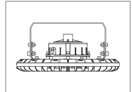
2. Screw the U-shaped bracket onto the bracket fixing plate.
