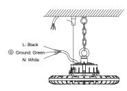
4. Connect the wire according to wiring diagram.
