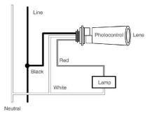
Do not install the switch with the Photocell facing artificial or reflected light. This will cause the unit to cycle on and off at night.
